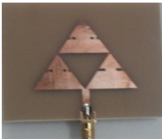
**Fig. 3 photograph of Fractal reconfigurable multiband communicating antenna for Cognitive radio**
